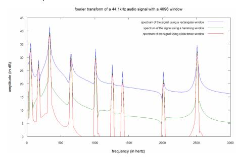
The signal is sampled at 44100Hz so a 4096-sample window represents a 93-millisecond part (4096/44100) and a frequency resolution of 10.7 Hz.
