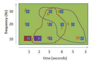
In this picture I plotted 2 target zones with their anchor points. Let's focus on the purple target zone. The address formula proposed by shazam is following one:
