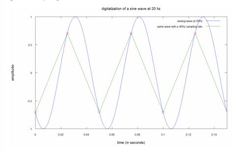
In this figure, a sound at 20Hz is digitalized using a 40Hz sampling rate:
