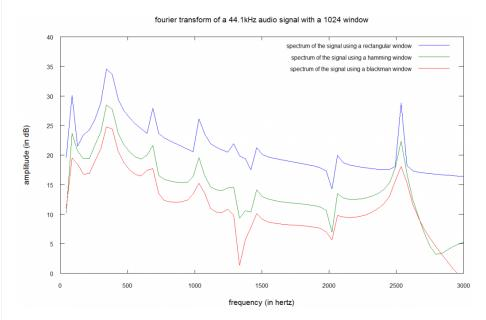
The signal is sampled at 44100Hz so a 1024-sample window represents a 23-millisecond part (1024/44100) and a frequency resolution of 43 Hz.
