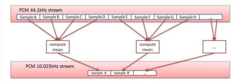
Downsampling a 44.1 kHz song to a 11.025 kHz one is not very difficult: A simple way to do it is to take the samples by group of 4 and to transform this group into just one sample by taking the average of the 4 samples. The only tricky part is that before downsampling a signal, you need to filter the higher frequencies in the sound to avoid aliasing (remember the Nyquist-Shannon theorem). This can be done by using a digital low pass filter.
