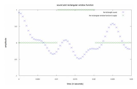
In this figure, to get the frequencies for the second 0.01-second part, you need to multiply the sampled audio signal (in blue) with the window function (in green).
