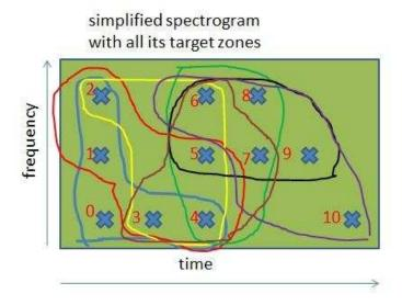
In this simplified spectrogram, you can see the different target zones generated by the previous algorithm. Since the target size is 5, most of the points belong to 5 target zones (except the points at the beginning and the end of the spectrogram).
