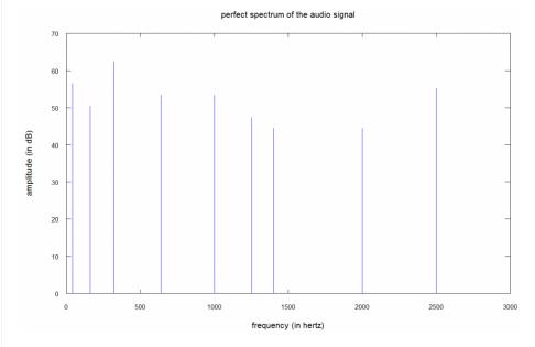
This figure shows a spectrum with only 9 vertical lines (at 40 Hz, 160 Hz, 320 Hz, 640 Hz, 1000 Hz, 1225 Hz, 1400 Hz, 2000 Hz and 2500 Hz. The y axis gives the amplitude in decibels (dB) which means the scale is logarithmic. With this scale a sound at 60 dB is 100 times more powerful than a sound at 40 dB and 10000 times more powerful than a sound at 20 dB. To give you an idea, when you speak in a quiet room, the sound you produce is 20-30 dB higher (at 1 m of you) than the sound of the room.
