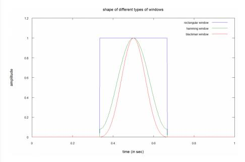
In this figure, you can multiply the audio signal with one of the 3 window types to get the part of the signal between 0.333sec and 0.666 sec. As I said, using a rectangular window is like cutting the signal between 0.333sec and 0.666sec whereas with the Hamming or the Blackman windows you need to multiply the signal with the window signal.
