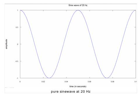
In this figure, you can see the representation of a pure sine wave of frequency 20hz and amplitude 1.
