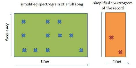
Visually speaking, I need to superpose the small spectrogram everywhere inside the spectrogram of the full song to check if the small spectrogram matches with a part of the full one.
