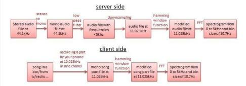
On the server side (Shazam), the 44.1khz sampled sound (from CD, MP3 or whatever sound format) needs to pass from stereo to mono. We can do that by taking the average of the left speaker and the right one. Before downsampling, we need to filter the frequencies above 5kHz to avoid aliasing. Then, the sound can be downsampled at 11.025kHz.
