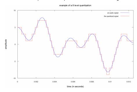
This figure presents an 8 level quantization. As you can see, the resulting sound (in red) is very altered. The difference between the real sound and the quantized one is called **quantization** error or quantization noise. This 8 level quantization is also called a 3 bits quantization because you only need 3 bits to implement the 8 different levels  $(8 = 2^3)$ .
