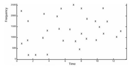
This figure (still from the Shazam research article) is a filtered spectrogram. Only the strongest frequencies from the previous figure are kept. Some parts of the song have no frequency (for example between 4 and 4.5 seconds).
