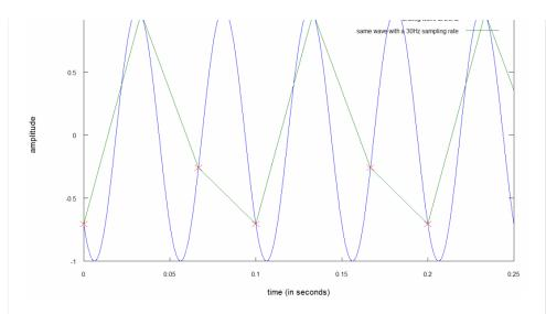
In this figure, a sound at 20 Hz is digitalized with a 30Hz sampling rate. This time the **frequency of the sampled signal is not the same as the original signal**: it's only 10Hz. If you look carefully, you can see that one cycle in the sampled signal represents two cycles in the original signal. This case is an under sampling.
